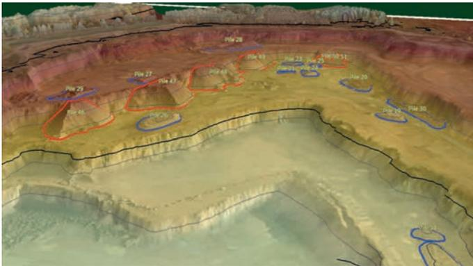
Drones provide the ability to quantify stockpiles quickly, accurately and without exposing personnel to potential risks. Photo courtesy of Hexagon Mining
