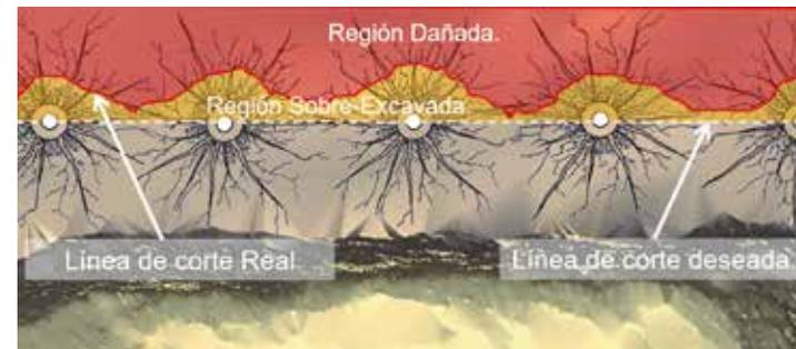
Idealisation of over-excavation and damaged region after blasting.
